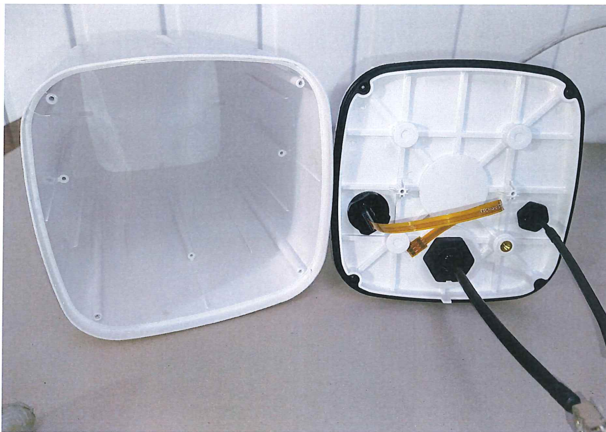
Fig. 7. View inside the enclosure after the IPX8 test
